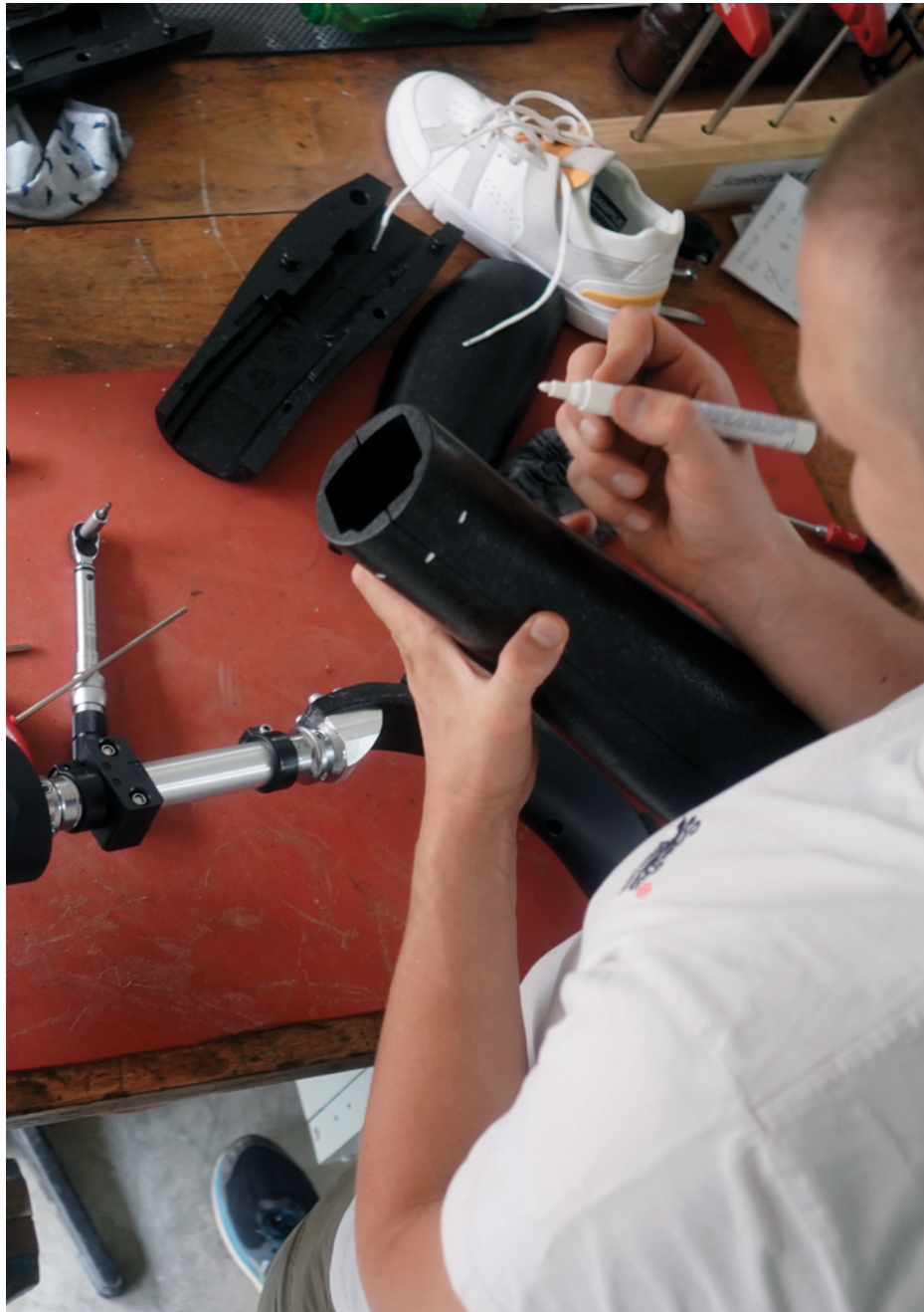
The Cosmetic Cover can be marked and shortened to each needed length with a simple saw or cutting knife
