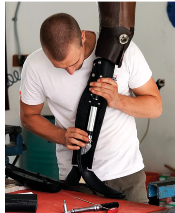
The Cosmetic Cover is clicked onto the Pylon Kit, making fitting fast and easy.
