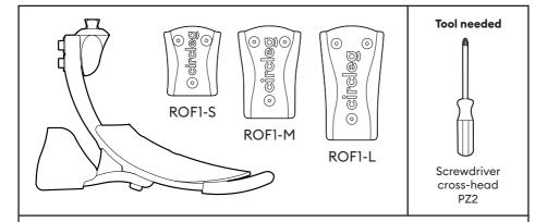
Mount the Sole Pad (ROFI) **after bench alignment** with a screwdriver to the pre-drilled holes on the Circleg Dynamic Foot.
