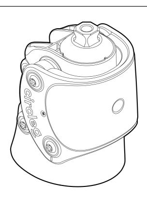
The Circleg polycentric knee provides a high level of stability at heel strike and good ground clearance during the swing phase. It has an extension assist spring and a flexion damper to reduce energy consumption and improve the gait cycle. The knee cap protects the mechanism from dirt. The Circleg polycentric knee allows up to 150 degrees of knee flexion. It can be used for amputations ranging from through knee amputation to a minimum femoral stump length of 10 cm.
