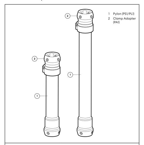
The Pylon Kit consists of an aluminium tube with a fixed stainless steel clamp adapter (PS1/PL1) and a screw-on Clamp Adapter (PA1) that allows 360° rotation. They connect the dynamic foot to the proximal components. The Pylon Kit allows for controlled angle and length adaptation in the sagittal and frontal plane and inward and outward rotation adjustment. The Pylon Kit comes in 250 mm and 400 mm sizes and is intended for a maximum body weight of 110 kg.
